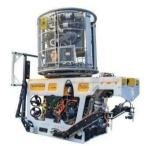
Top Hat Tether Management System with 350m capacity of 20mm tether, fitted with latch status and line out sensors. Options include depth and current sensors, and additional downward looking light and camera.
